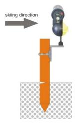
Photocell system A and B must always be completely separate (separate case and mounting brackets).
