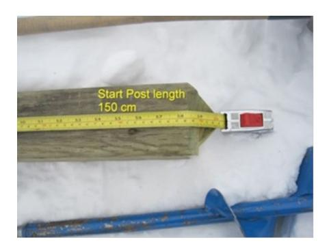
The start gate consists of two square posts, 150cm long and 9cm square. The top of the posts must be flat. The posts must be placed at the front edge of the start ramp. The area up to the front face of the posts must be level. The slope starts at the front face (course side) of the posts.
