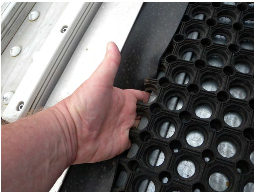
only floppy rubber covers rails of ice moulding machine
