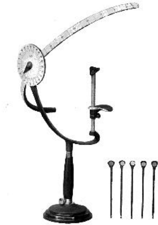
Figure 2 Hand-held arc perimeter for the measurement of visual field
