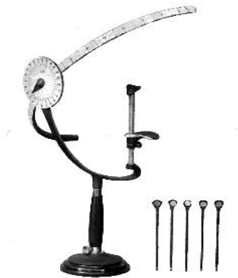
Figure 2 Hand-held arc perimeter for the measurement of visual field
